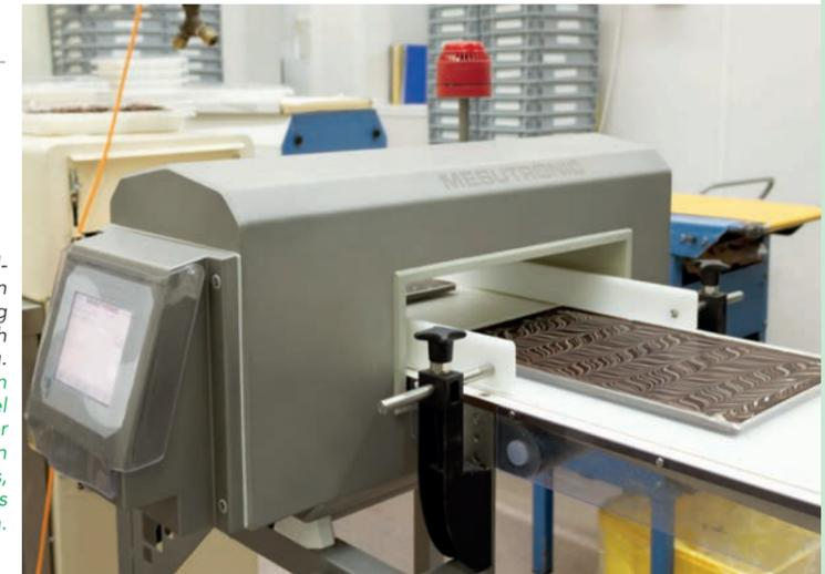
such as the plastics or textile industry, the devices are mainly used for machine protection, in the food or pharmaceutical industry mostly for quality control.
