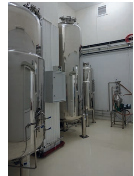
Anlage zur Gewinnung hochwertiger thermostabiler Phytase-Enzyme. Fermentor for the production of high quality thermostable phytase enzymes.
