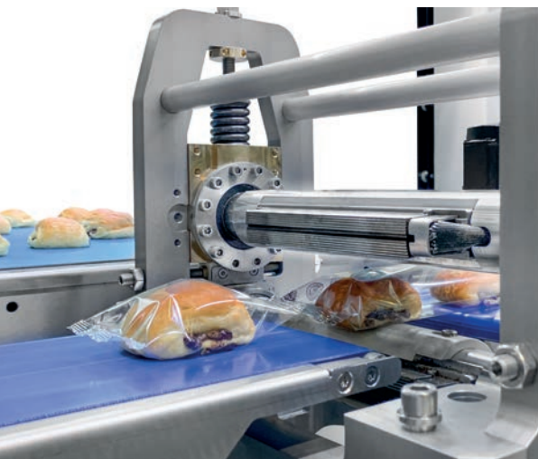
Der Flowpacker verpackt alle Arten von Backwaren in Schlauchbeutel. (Bilder: Gerhard Schubert GmbH) The Flowpacker efficiently packs all types of baked goods into flowpacks. (Images: Gerhard Schubert GmbH)
